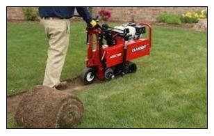
Set the depth of the cutting blade on the sod cutter following the manufacturer's instructions.
